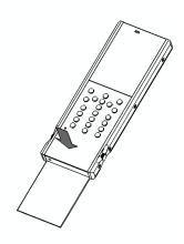
Insert the SIM card. Make sure the golden contact area is facing downwards and is oriented as shown.
