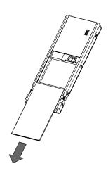
Remove the battery by turning the phone over and gently knock against the palm of your hand until the battery comes out.
